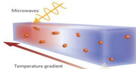
Innovative concept of applying high frequency electromagnetic energy to substance which results in to generation of heat within material without applying heat from outside. When the material to be heat is subjected to high frequency electromagnetic field, the water molecules in the material reorient constantly to align with the changing field. This movement generates heat inside water molecules and makes entire mass of water to evaporate uniformly.
